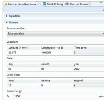
Defining an external radiation source using the Solar Position option.
