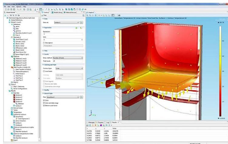
Analyzing heat transfer in a two-floor structure with a thermal bridge.
